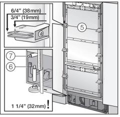
The installation aids (5) on the appliance door have been designed for the following custom door thicknesses:
